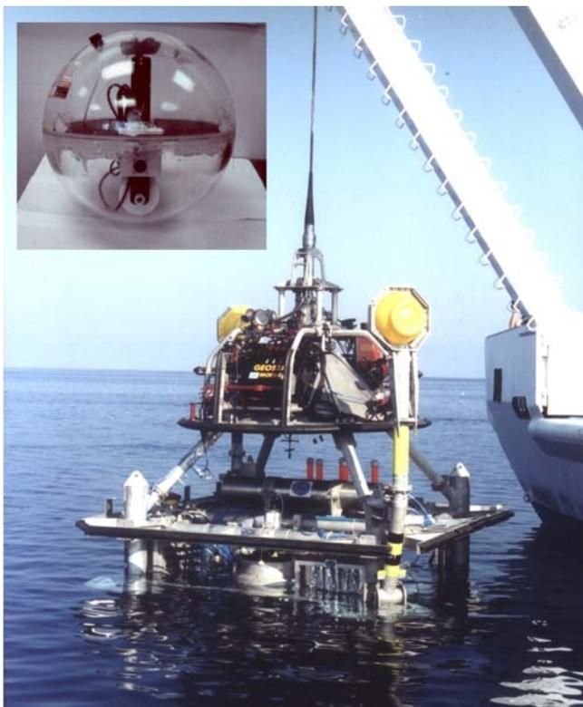
Figure 1.7: Mobile docker and seafloor station used in the framework of GEOSTAR (Geophysical and Oceanographic STation for Abyssal Research) European Project. The GEOSTAR sea bottom observatory contains several sensors, among them a scalar Overhauser magnetometer and a three-component suspended flux-gate magnetometer, both placed in the yellow boxes at the end of the two booms, which are extended at the seafloor (Courtesy of A. De Santis).
